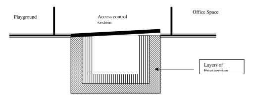
Example of a sketch of pit type storage facility is shown above. For cabinet storage or walled building, sketch the housing facility appropriately.
