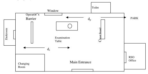
Sketches of storage facilities should specify the access control system and the distances of occupancy from the sources. Also state the materials and the different levels of barriers.
